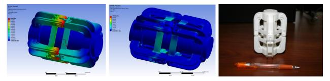
ANSYS simulation of the torque sensor behaviour under the action of centrifugal force at 10.000 rpm. Left: radial displacement; Middle: von Mises stress; Right: Beta version of the torque sensor
